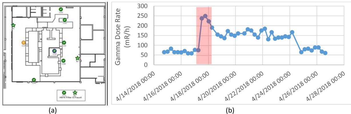
Figure 5. ARG-US RFID tags and readers in AGHCF (a) and (b) gamma dose rate data for RFID Tag #5210 inside Clean Transfer Area (CTA).
