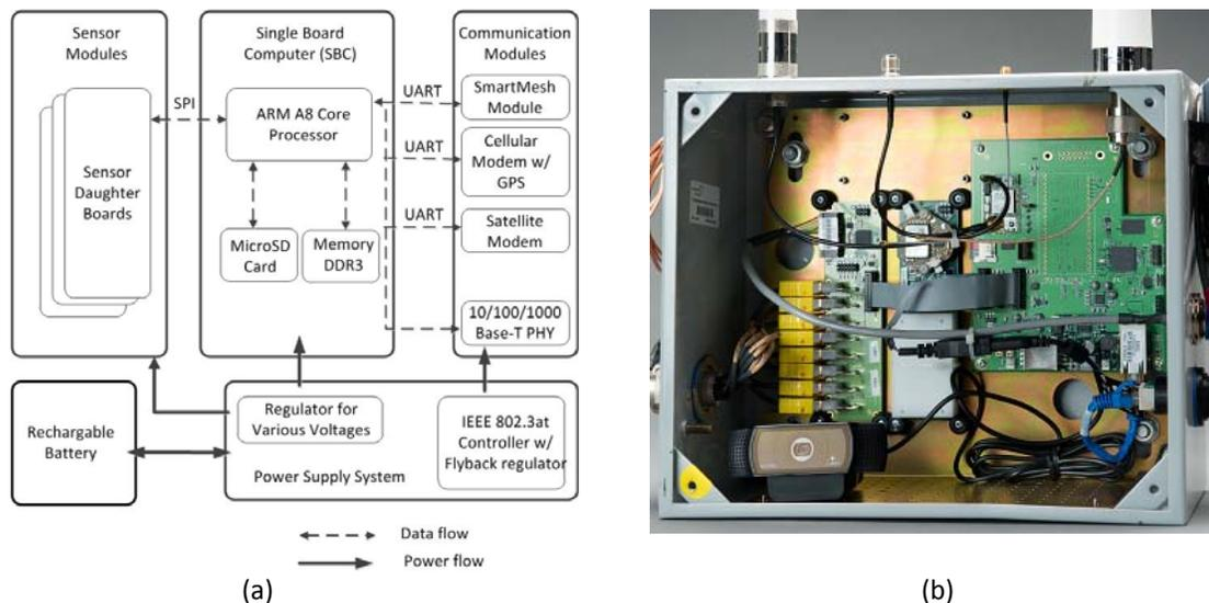
Figure 1. Block diagram of remote area modular monitoring (RAMM) (a), with a digital camera mounted on the base inside the lunch-box-sized unit (b).
