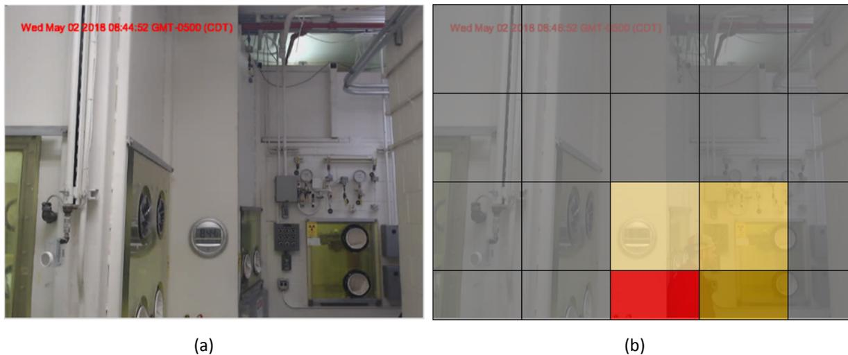
Figure 7. (a) Camera image from Unit #1114 before motion (event) detection on May 02 2018 08:44:52 GMT and (b) pixel-frame-based motion (event) detection on May 02 2018 08:46:52 GMT. (Colors indicate differences in changes of image intensities in successive images.)
