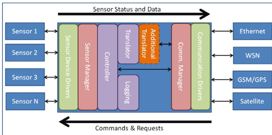
**FIGURE 4. Block diagram of the onboard RAMM software**
