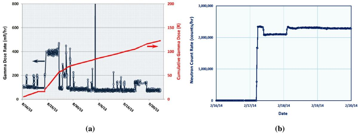
**FIGURE 3. Sample radiation sensor performance in a radiological Facility: gamma (a) and neutron detectors (b)**
