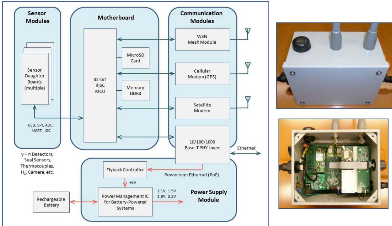
**FIGURE 2. Block diagram and a pre-construction prototype of a RAMM unit**
