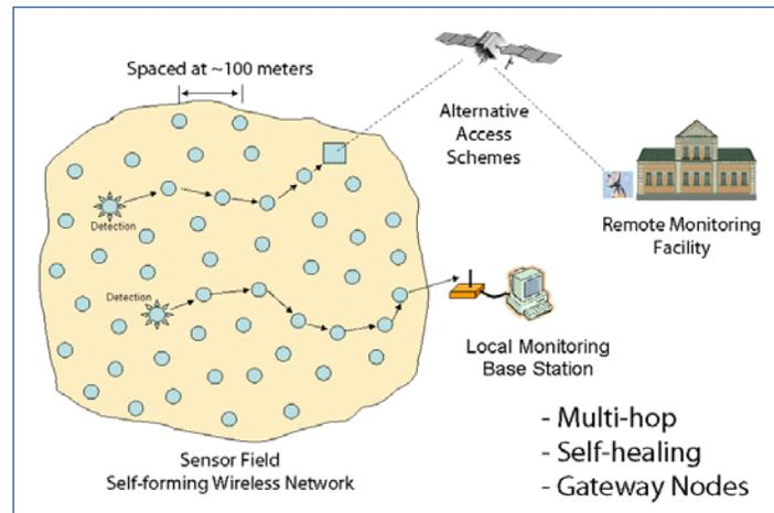
**FIGURE 1. Mesh wireless sensor network for RAMM**
