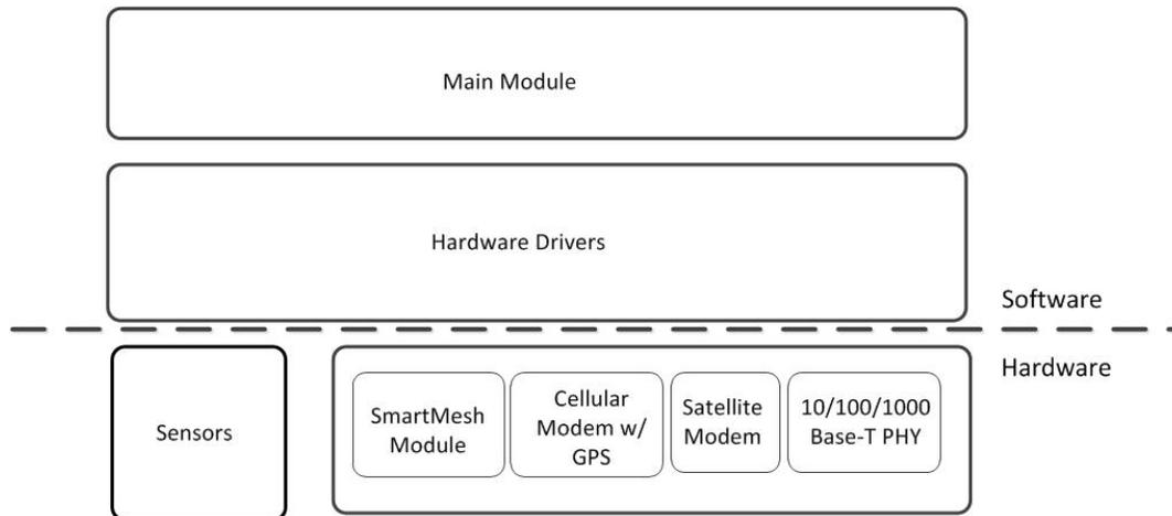
Figure 4. Application software architecture and hardware interface of a RAMM unit
