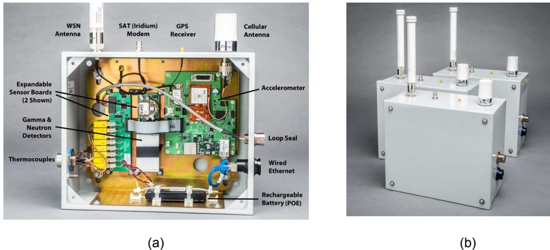
Figure 1. (a) RAMM unit, shown with interior exposed, and (b) closed view of contractor-manufactured RAMM units, shown without external connections
