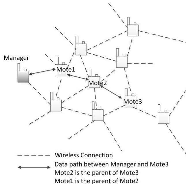
Figure 3. Schematic of a SMIP WSN consisting of one Manager and multiple Motes.
