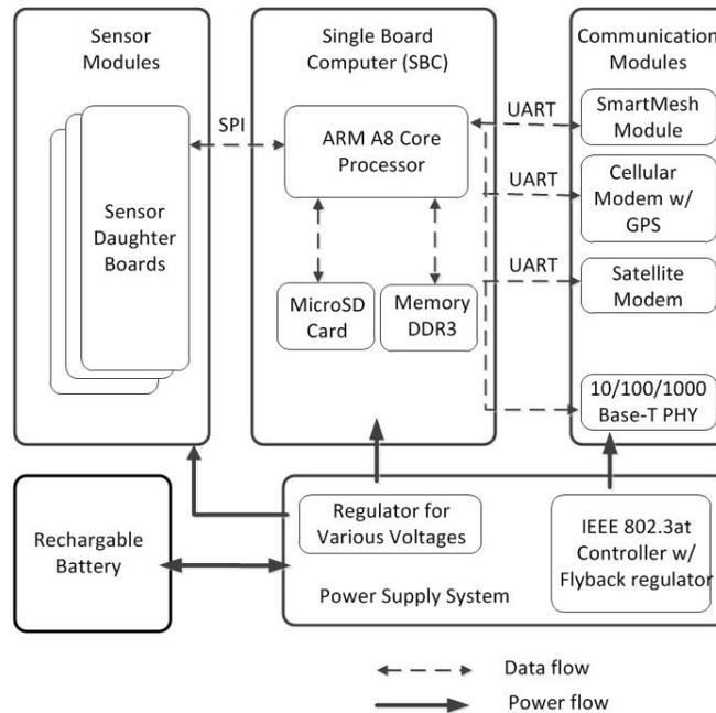
Figure 2. Block diagram of hardware architecture design of a RAMM unit
