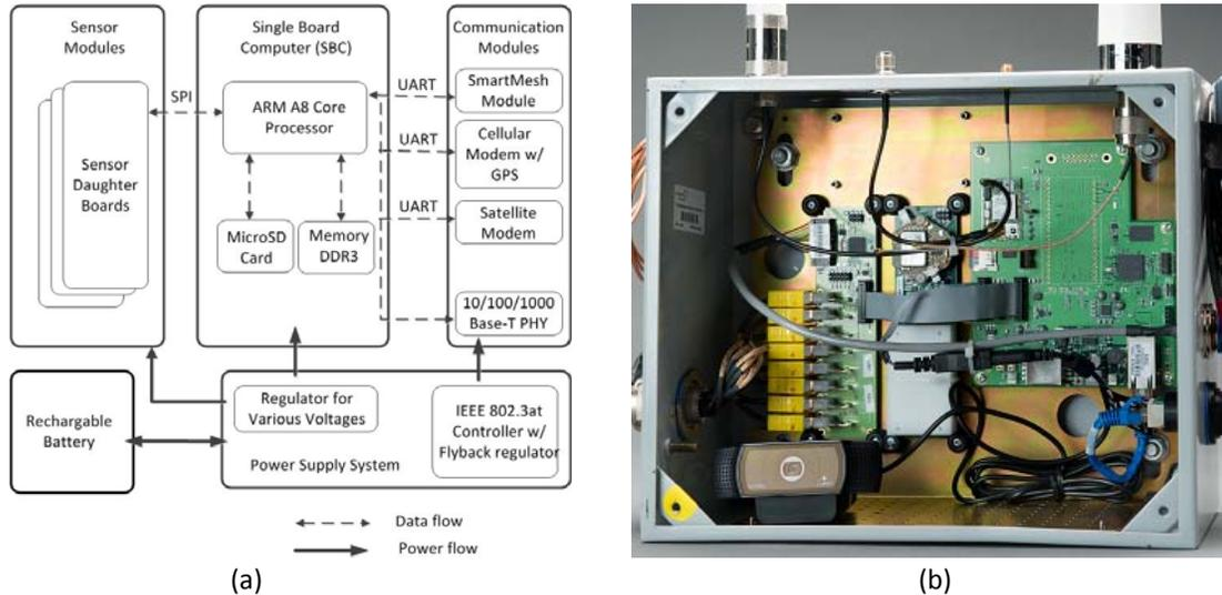
Figure 1. Block diagram of a RAMM unit (a), and its prototype embodiment incorporating a digital camera and other sensors inside the lunch-box-sized unit (b).
