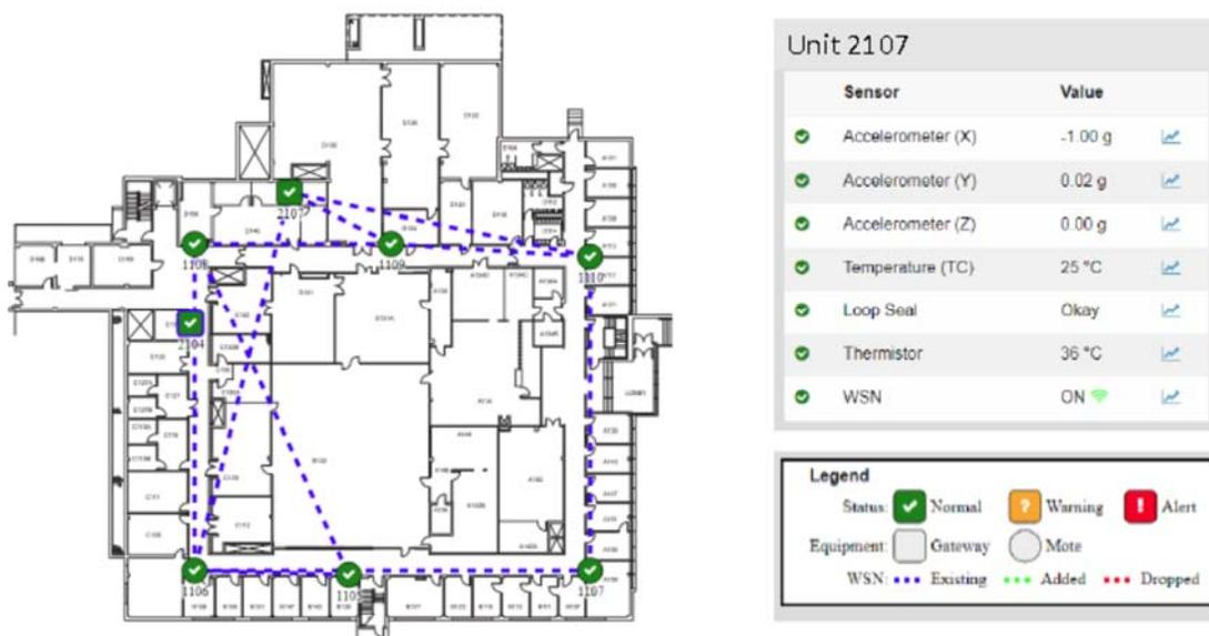
Figure 3. RAMM units deployed on the first floor of an office building: six Motes and two Managers (only #2107 was enabled; #2104 is a standby) on 10 May 2019, 21:27:25 GMT.
