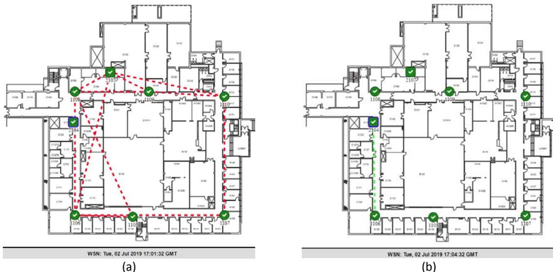
Figure 5. Switching between Managers (gateways) #2107 (a) and #2104 (b) for a WSN of RAMM units. Radio links (red) between Manager #2107 and the Motes were dropped in (a), whereas the first radio link (green) between Manager #2104 and Mote #1106 was added in (b).
