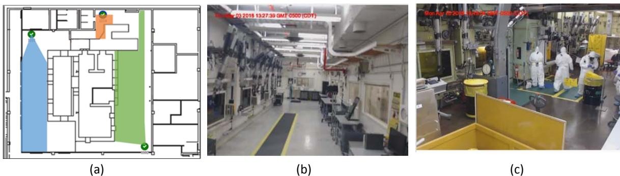
Figure 2. RAMM units with digital cameras in the AGHCF: (a) accessible areas shaded to show coverage by Units #1101, #1102 and #1114; (b) camera image of front entry taken by Unit #1101; and (c) camera image of CTA taken by Unit #1102.
