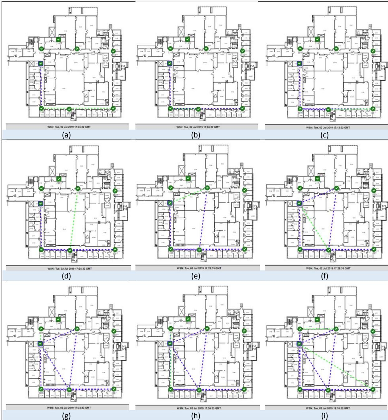
Figure 6. Self-forming sequence (a) to (i) of WSN of RAMM units (Motes) following switch to Manager #2104.
