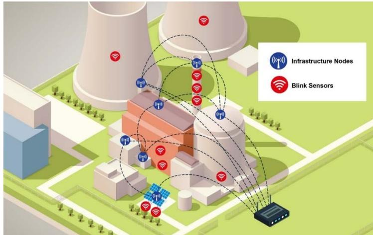
Figure 2. Schematic illustrating facility monitoring using wireless sensors network of RAMM (infrastructure nodes) and blink sensors
