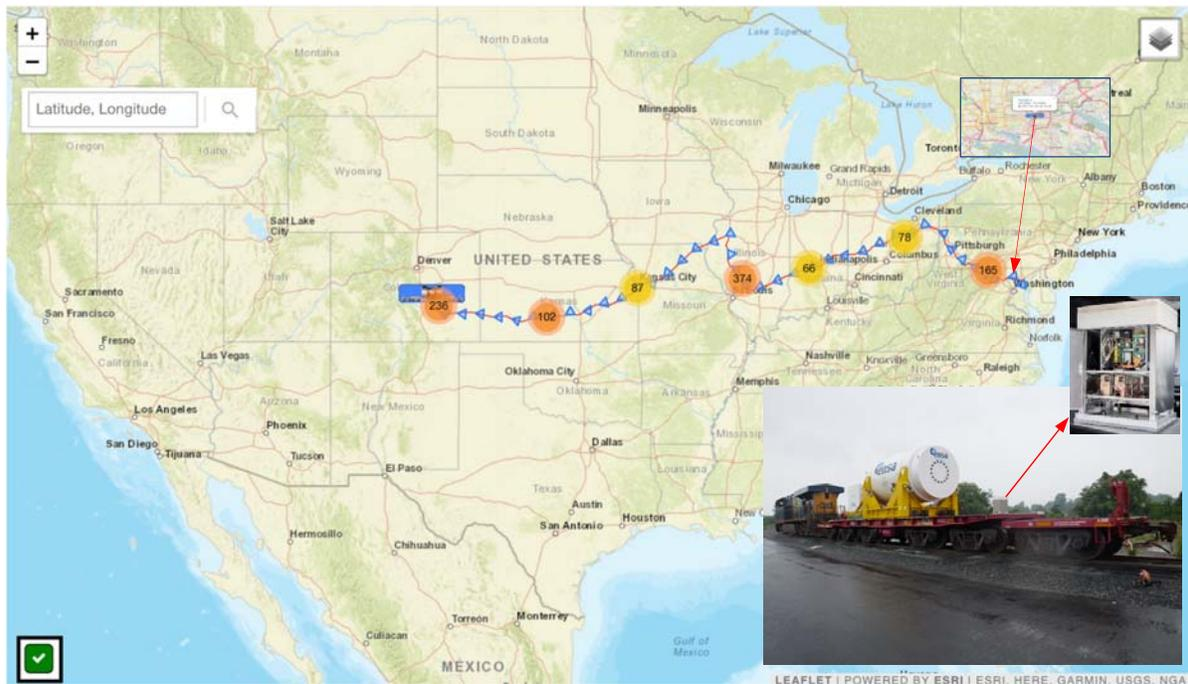
Figure 6. Iridium satellite tracking the ENSA/DOE transport cask as it is shipped by rail from Baltimore, Maryland, to Pueblo, Colorado, from July 28 to August 3, 2017.
