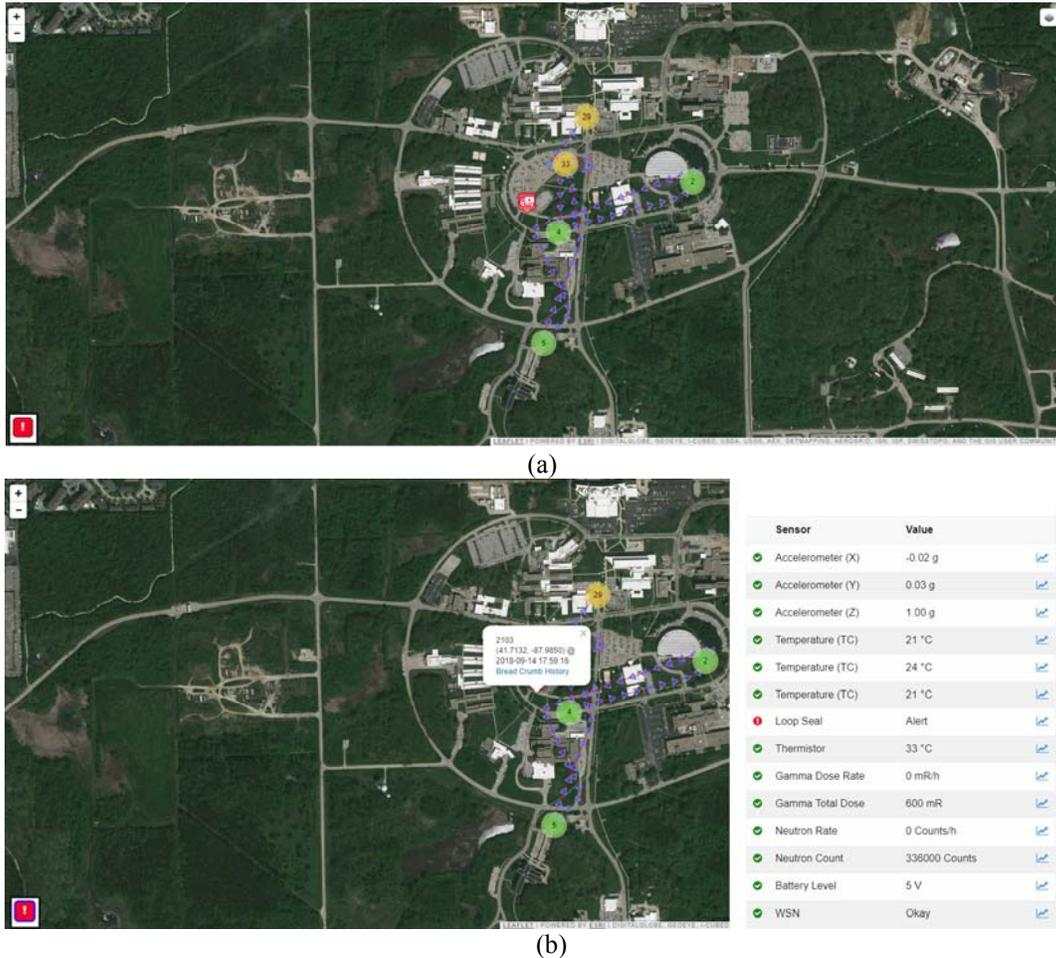
Figure 7. Loop seal alarm via cellular communication during TRAVELER's vehicle road test on the Argonne campus, September 14, 2018
