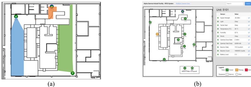
Figure 3. Floor views of Argonne’s radiological facility showing locations and coverage areas of (a) RAMM units (1101, 1102, and 1114) with digital video cameras, and (b) RFID surveillance tags (circles) and readers (stars).
