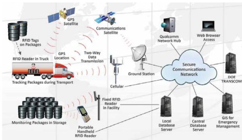
Figure 1. ARG-US RFID monitoring and tracking drum-type packages of radioactive materials during storage and transport
