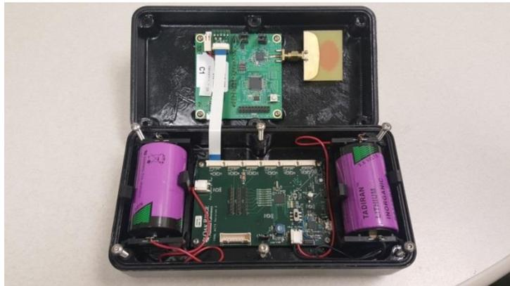
**Figure 2. ACTS test units incorporate the DecaWave EVK 1000 Ultra-wideband module to perform IEEE 802.15.4-2011 communications.**
