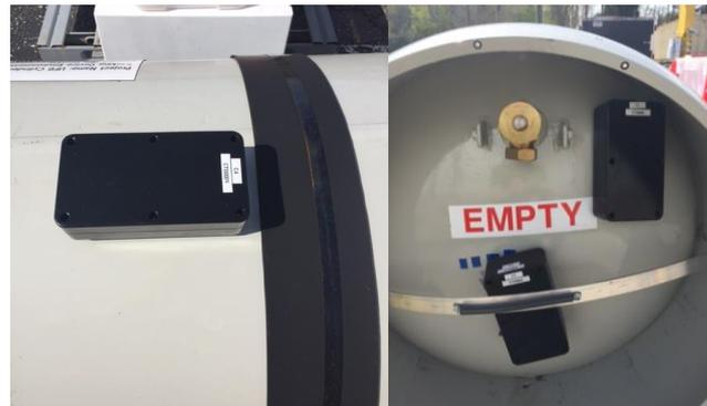
**Figure 8. Outdoor 30B container device placement**
