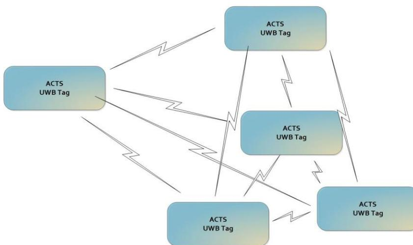
**Figure 4. Relative ranging between tags lets each tag determine the distances to neighboring tags and identify relative movements.**
