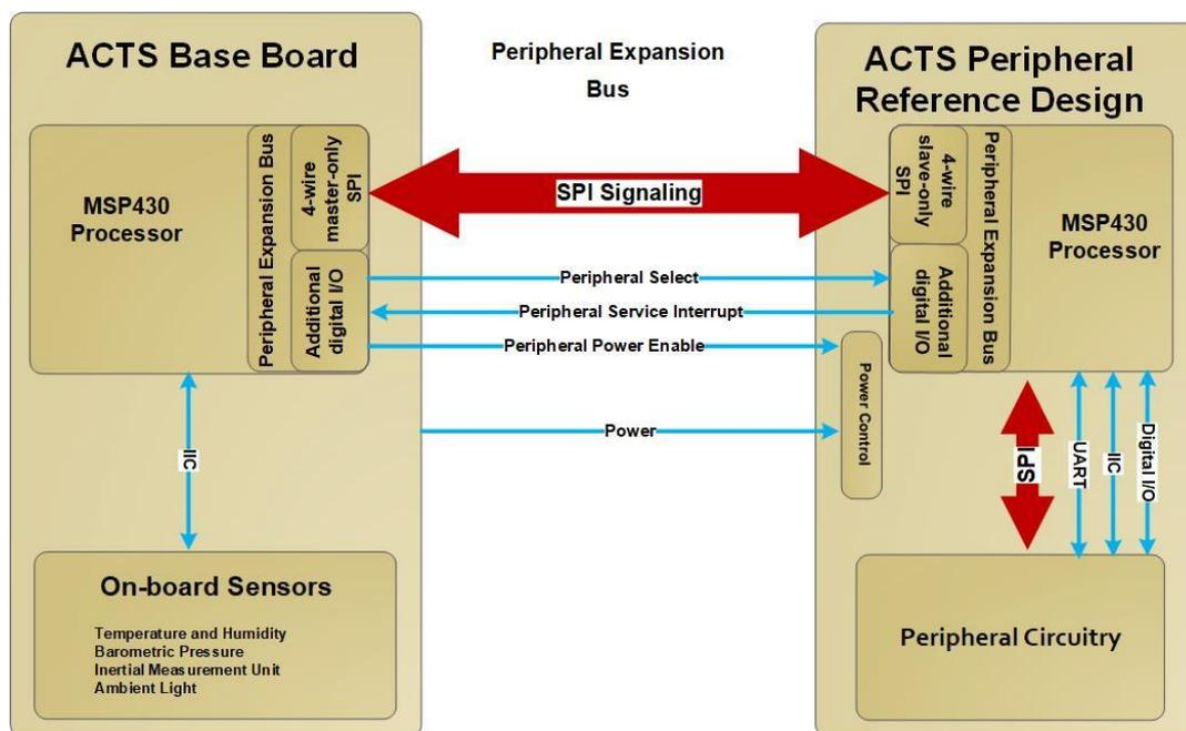
Figure 2. The ACTS base board architecture, built on the low-power MSP family of processors, incorporates a base set of relevant sensors and a peripheral interface for matching ACTS to specific applications.
