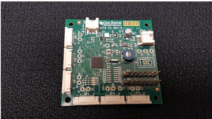
Figure 1. The size of the ACTS base board has been significantly reduced.
