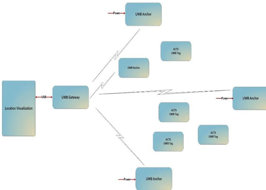
**Figure 3. Infrastructure-based ranging to locate items uses an infrastructure of anchor transceivers at known locations and a visualization system to show tagged assets.**
