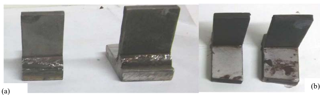
FIG. 54. Welded samples (WS) before (a) and after (a) surface cleaning (courtesy of CNEA).
