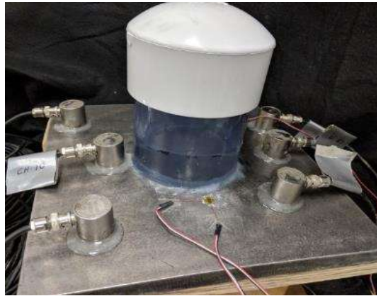
FIG. 47. Acoustic emission testing of a growing SCC flaw (courtesy of EPRI).
