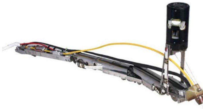
FIG. 38. Snake robotic platform proposed for the inspection of dry storage canisters (courtesy of EPRI).
