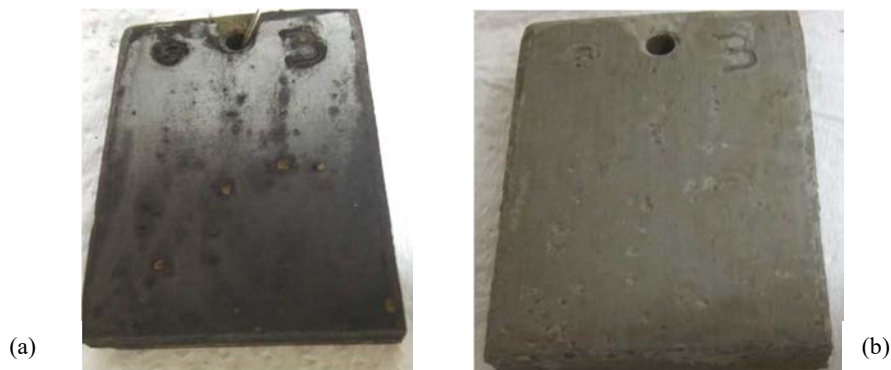
FIG. 53. CS coupon after test before (a) and after (b) surface treatment (courtesy of CNEA).
