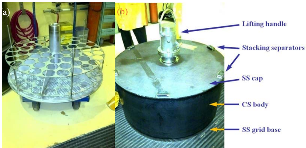
FIG. 24. (a) Stainless steel grid to hold spent fuel bundles from CNE. (b) Closed canister (courtesy of CNEA).
