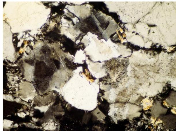
Fig. 2. Thin section of granite S93/7 after melting at 800°C and cooling to 560°C. (Cross polars. Field of view is ~1.2 mm wide.)
