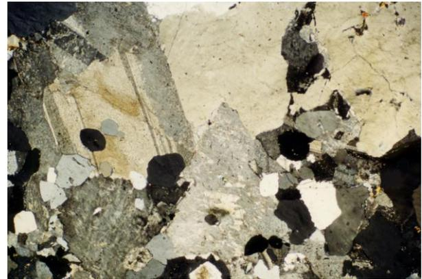
Fig. 1. Thin section of granite S93/7<sup>10</sup>. (Cross-polars. Field of view is ~5.5 mm wide).
