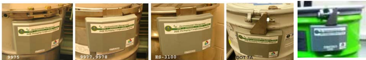
Figure 2. ARG-US RFID tags mounted on certified Type B (9975, 9977, 9978, and ES-3100), DOT 7A, and Type AF 9979 transportation packages (from left to right).
