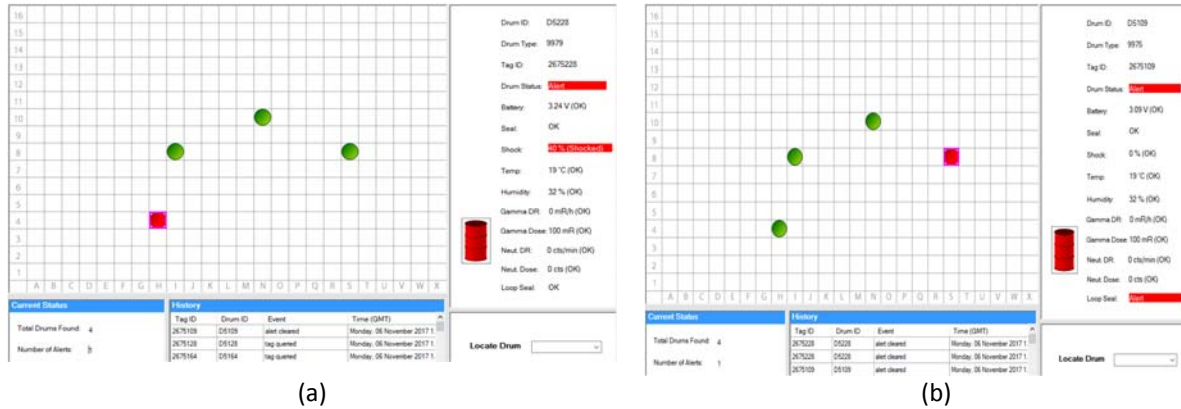
Figure 5. Screen shots of the State of Health of four tagged drums in the CC: (a) shock sensor alarm for 9979 and (b) loop seal alarm for 9975 [The loop seal is shown attached to the RFID tag in Fig. 4(c)]
