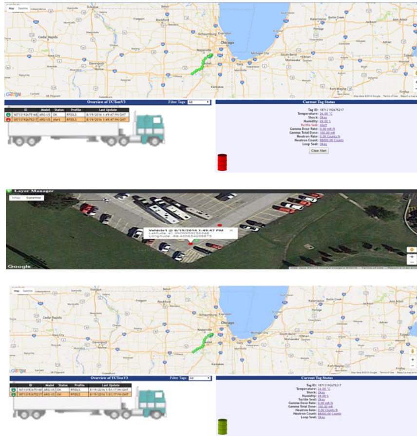
Figure 6. Screen shots of the tactile seal alarm sent by the RFID tag (#5217, top); satellite view of the time stamp and geographical location (latitude and longitude) of the vehicle/alarm in a parking area (middle); and after the tactile seal alarm was cleared at 1:51:17 pm GMT, August 19, 2016 (bottom).
