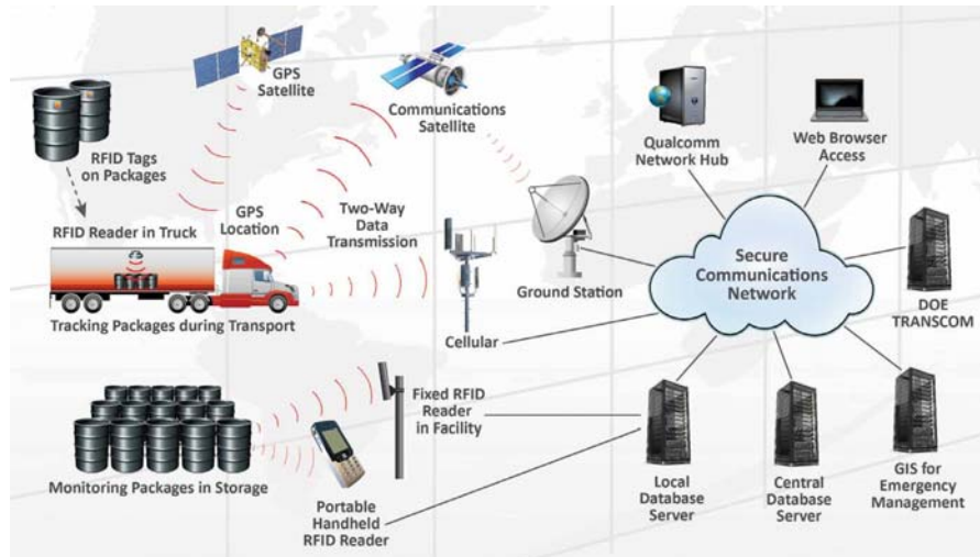
Figure 8. Application of ARG-US RFID system for drum-type packages in storage and transportation.
