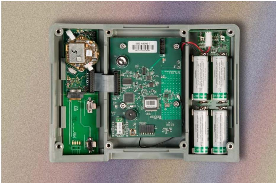
Figure 1 – Interior view of an ARG-US RFID tag, with the metal back plate and seal sensor removed
