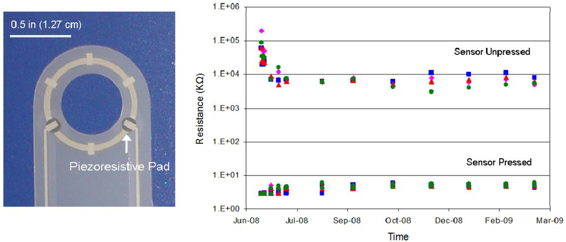
**Figure 4. Performance testing of seal sensors for the 9977 drums. Applied torque was 45 ft·lb (60.75 N·m) and the test employed four duplicate sensors.**
