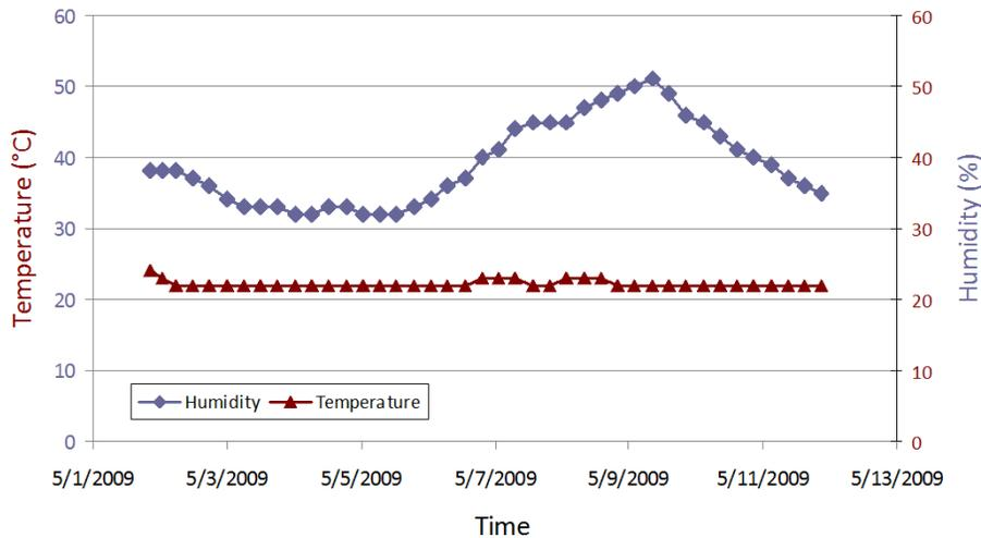
**Figure 5. Typical sensor data of Mk-2 tags monitored by ARG-US OnSite (6-hour interval).**
