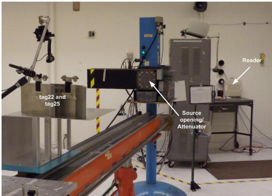
Figure 5. Irradiation testing of two dosimeter-enabled tags, Tags 22 and 25, mounted on a platform at an equal distance from the Shephard Cs-137 source.
