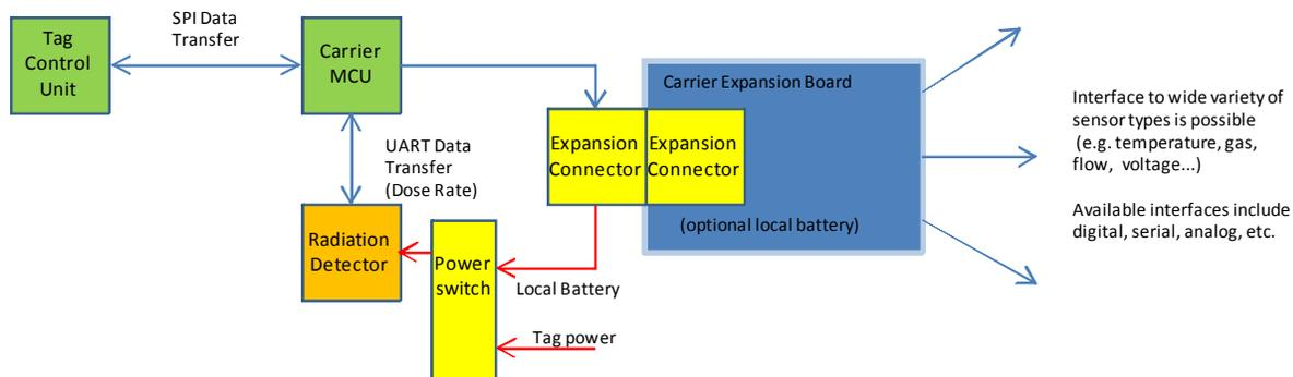
Figure 4. Block diagram of the dosimeter carrier board showing communication between the radiation detector (dosimeter), the MCU on the carrier board, and the tag control unit on the tag controller board.
