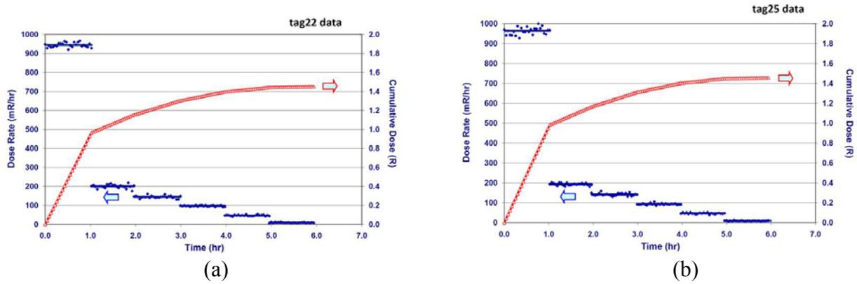
Figure 6. Results from 60-minute irradiation tests of (a) Tag 22 and (b) Tag 25 at target and intermediate dose-rate levels (from left to right: 1,000, 200, 150, 100, 50, and 10 mR/h). Horizontal straight blue lines are the averaged values of the measured dose rates.
