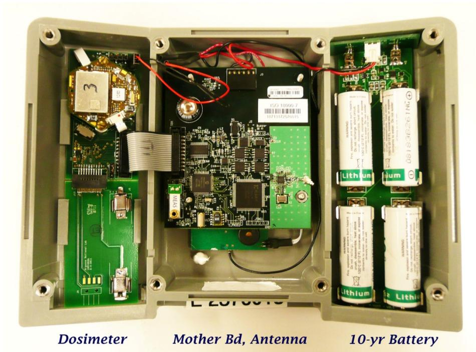
Figure 3. MK-III tag with a dosimeter carrier board incorporated in the left compartment.
