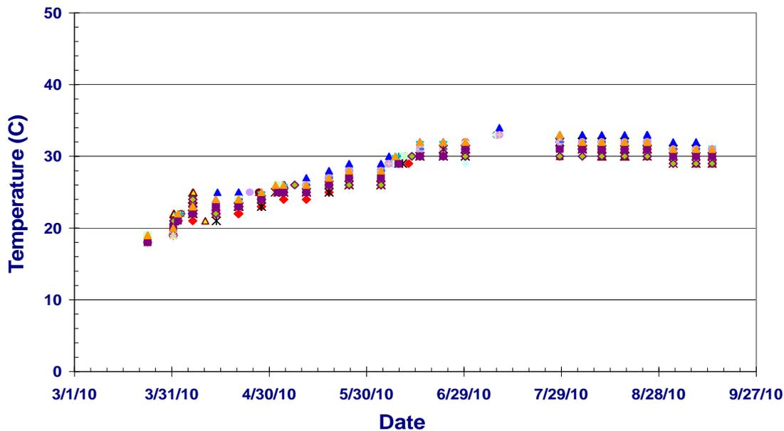
Figure 8. Aggregated temperature data for 20 MK-II tags distributed in a Category 1 vault over a period of  $\approx 6$  months. The system was not available during several weeks in July 2010.
