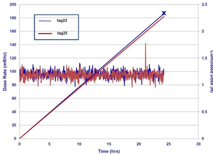
Figure 7. 24-h irradiation test results for Tags 22 and 25 at 100-mR/h. The “blue star” at the end of irradiation is the reading of a certified dosimeter standard.
