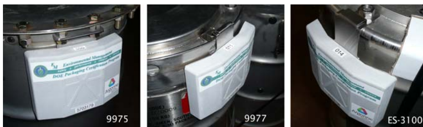
RFID tags mounted on Models 9975, 9977 and ES-3100 drums
