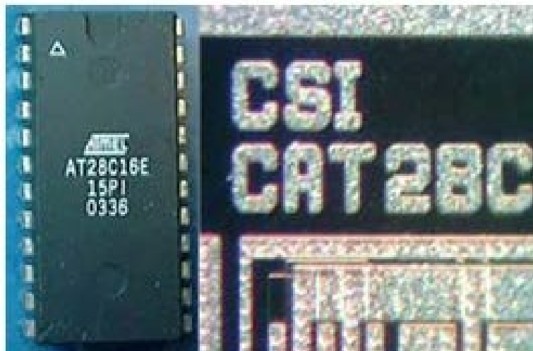
Figure 16: Counterfeit Atmel Device
