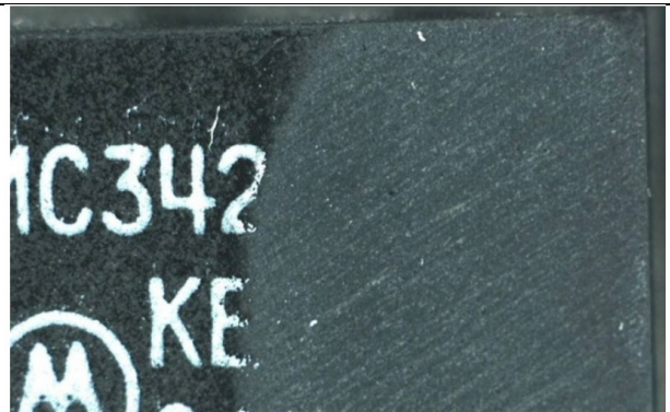
Figure 22: Example Resistance to Solvent Failure
