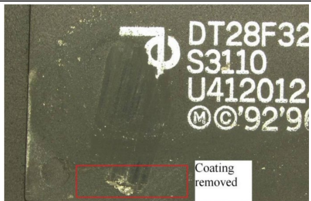
Figure 23: Example Scrape Test Failure
