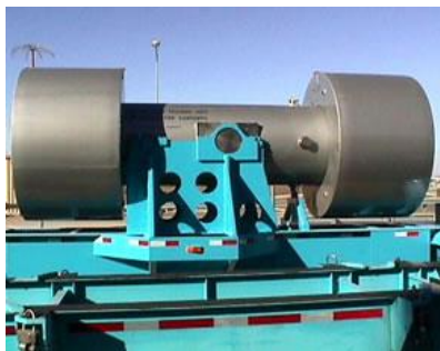
Figure 2 – RH-72B Container Loaded on a Trailer
