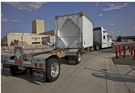
Figure 3 – TRUPACT-III Container Loaded on a Trailer
