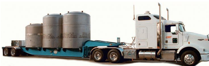
Figure 1 - Transport Vehicle with Two TRUPACT-II Containers and One HalfPACT Container.
