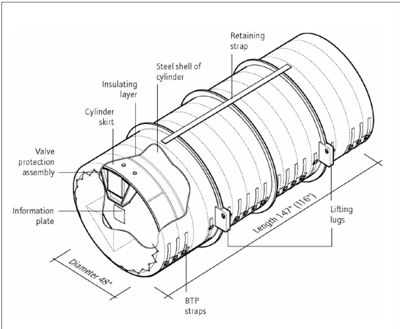
48Y (48X) UF<sub>6</sub> Cylinder (with Blanket Thermal Protector) (all dimensions are approximate)
